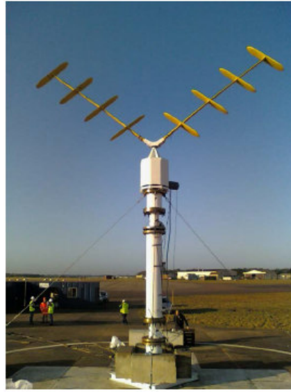
Figure 1. 5kW prototype device developed by Wind Power Ltd [6]
