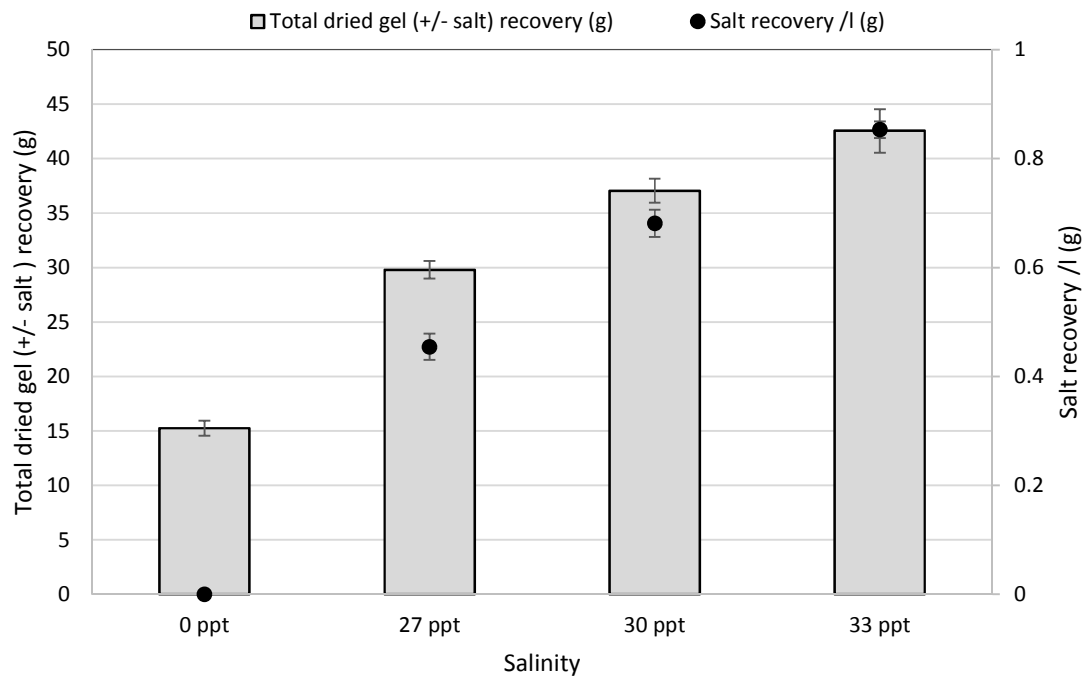
Figure 5-6 Gravimetric Alginate/Salt Composite Recovery (g) from 16 l batches of artificial seawater
