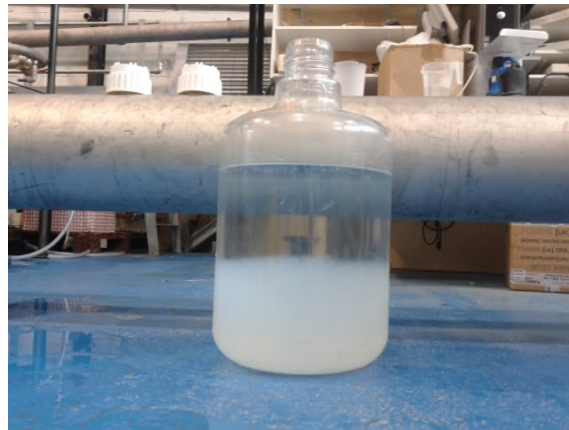
Figure 5-5 Density phase separation of gelled alginate in 33 ppt saline
