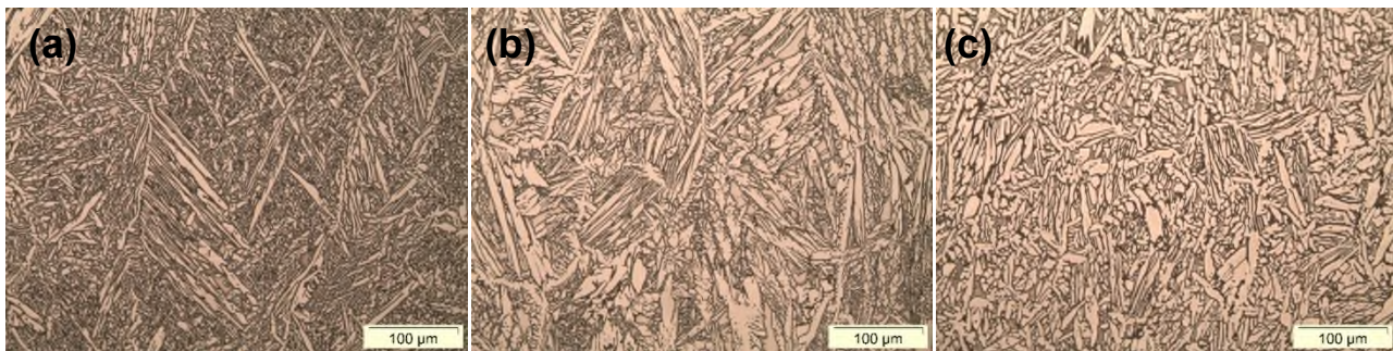
Figure 1: Root weld microstructure of (a) 100% Ar, (b) Ar + 2% N 2 and (c) 100% N 2 . The ferrite phase is here dark and austenite bright
