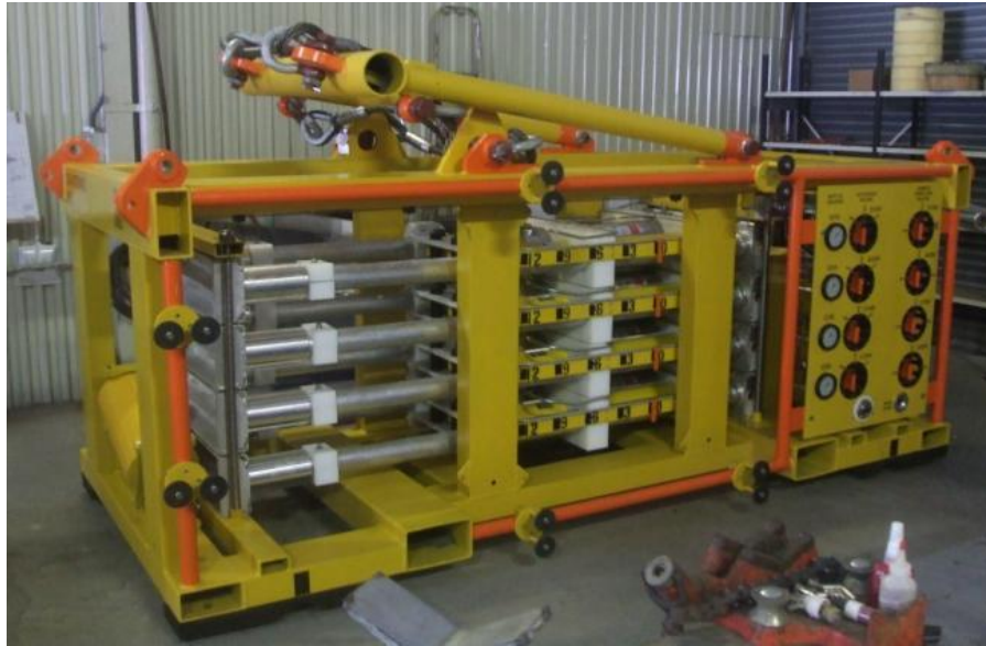
Figure 2-23 Subsea Fluid Sampling System (Source: Proserv)
