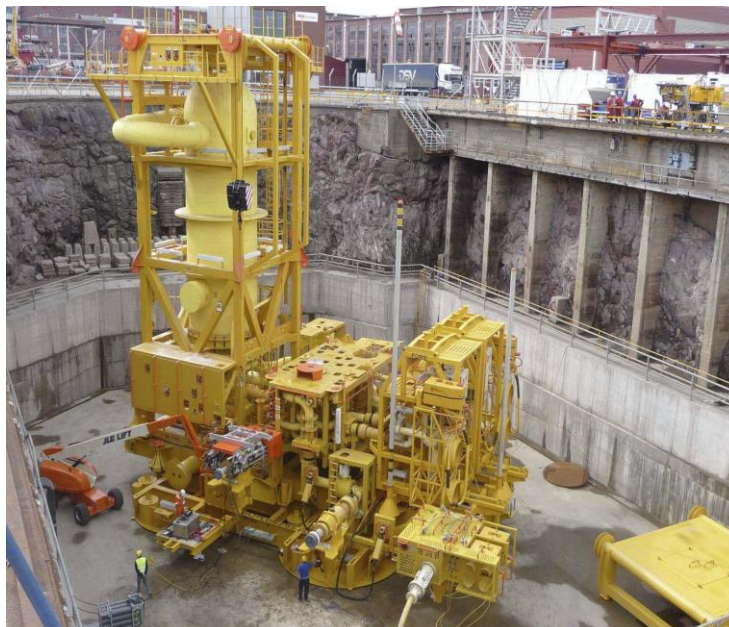
Figure 5-19 – Subsea Separation System for Maximized Recovery (Source: FMC)
