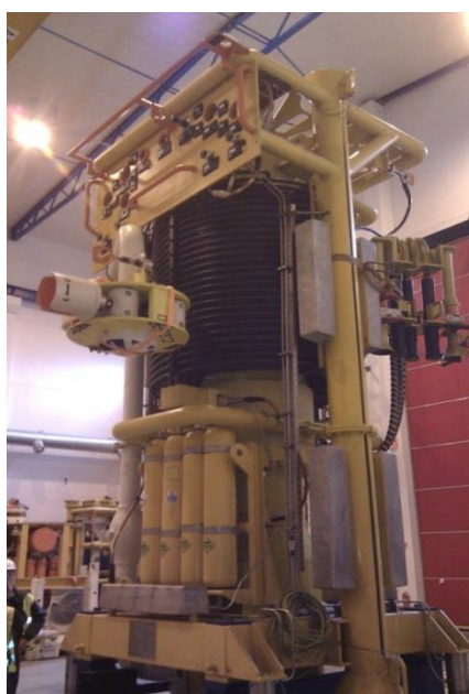
Figure 5-19 – Subsea Separation System for Maximized Recovery (Source: FMC)
