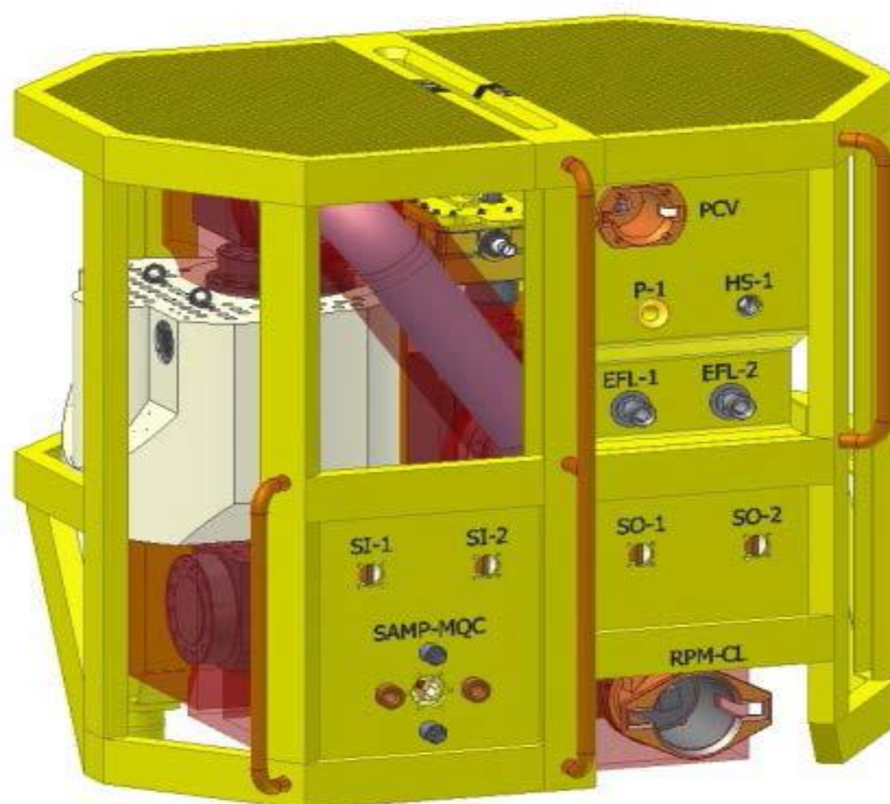
Figure 2-28 Dedicated Fluid Sampling FCM with Sampling Stab Plate (Source: Deepwater project)
