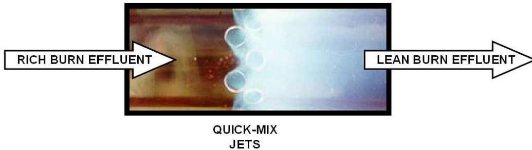
Figure 2-32: Laboratory Model of RQL Combustor [88]
