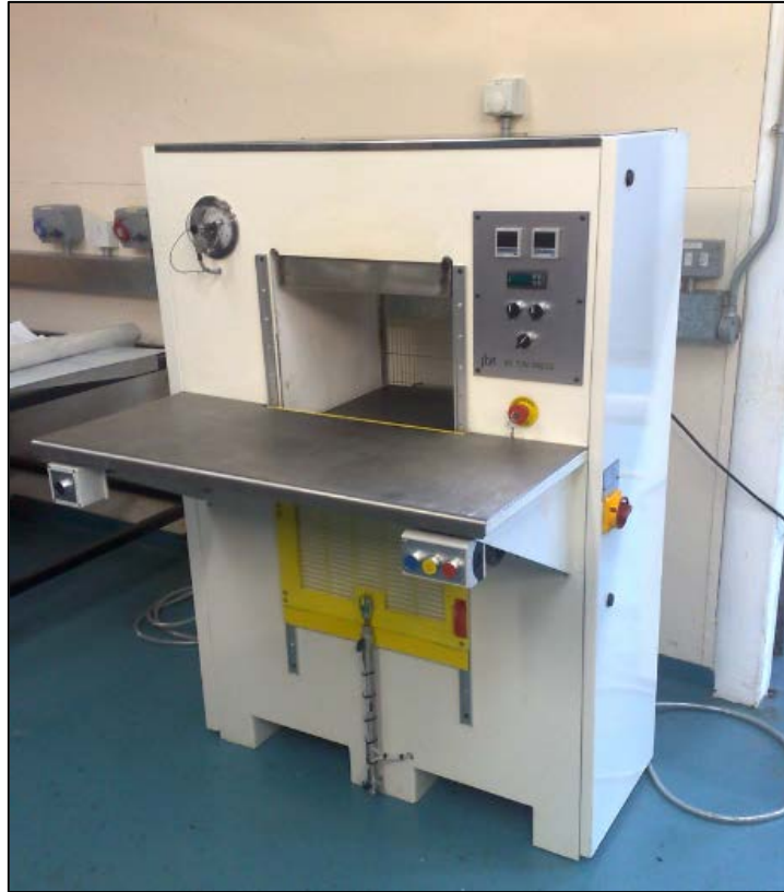
Figure 5-8 - JBT Engineering 40 tonne heated platen press
