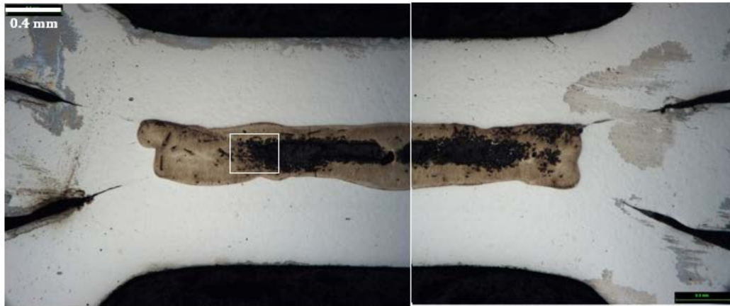
5.2 bar, 75 cycles (1.5 sec), 26% power (16.6 kVA) Specimen 120830-08
