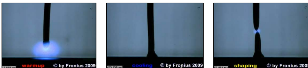
Figure 3-2 – Fronius CMT-Pin pike-head shaped micropin manufacture (Furukawa, 2006)
