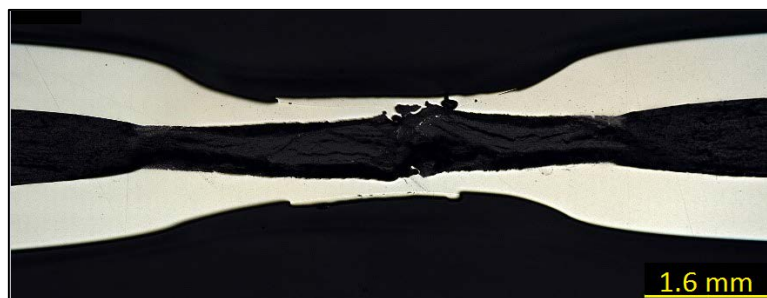
Figure 4-21 - Microsection of resistance spot weld trial of four plies of carbon fabric between sheets of 0.9mm thick stainless steel, welding parameters: 9kW for 1 seconds (9kJ)
