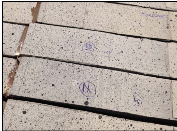
Figure 3-19 - Example of the speckled pattern required for Digital Image Correlation technique of surface strain visualisation
