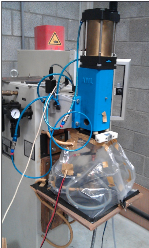
Figure 4-5 - AWL-Techniek WP63RL-K resistance spot welder, with gas enclosure tent around electrodes
