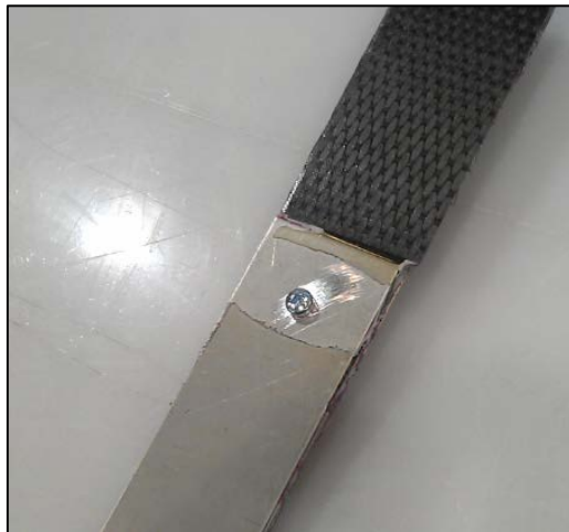
Figure 4-44 - Traditional reinforced adhesive joint; bolt of similar diameter as resistance welds installed on cured adhesive joints
