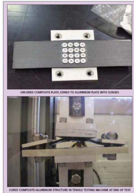
Figure 2-6 - Array of screws joining CFRP laminate to an aluminium plate; connection made prior to laminate cure. This was subsequently subjected to a tensile/bending test. Taken from (Semmes, 2009)
