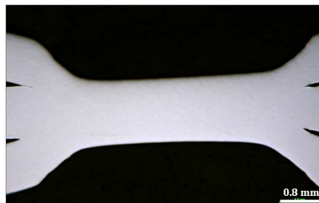
5.2 bar, 15 cycles (0.3 sec), 40% power (25.6 kVA) Specimen 120803-16
