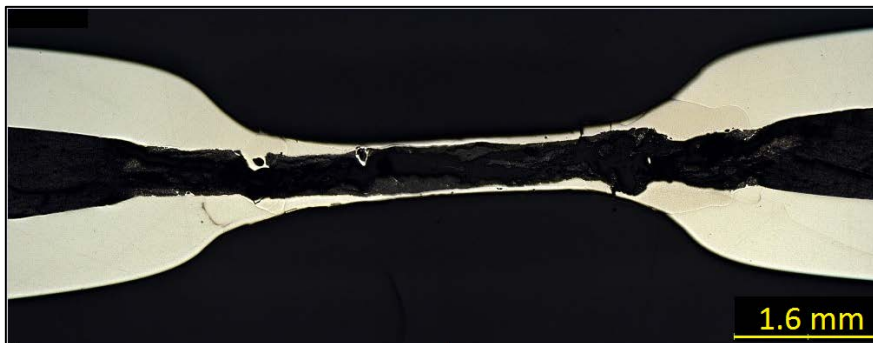
Figure 4-24 - Microsection of resistance spot weld trial of four plies of carbon fabric between sheets of 0.9mm thick stainless steel, welding parameters: 7kW for 2 second (14kJ).
