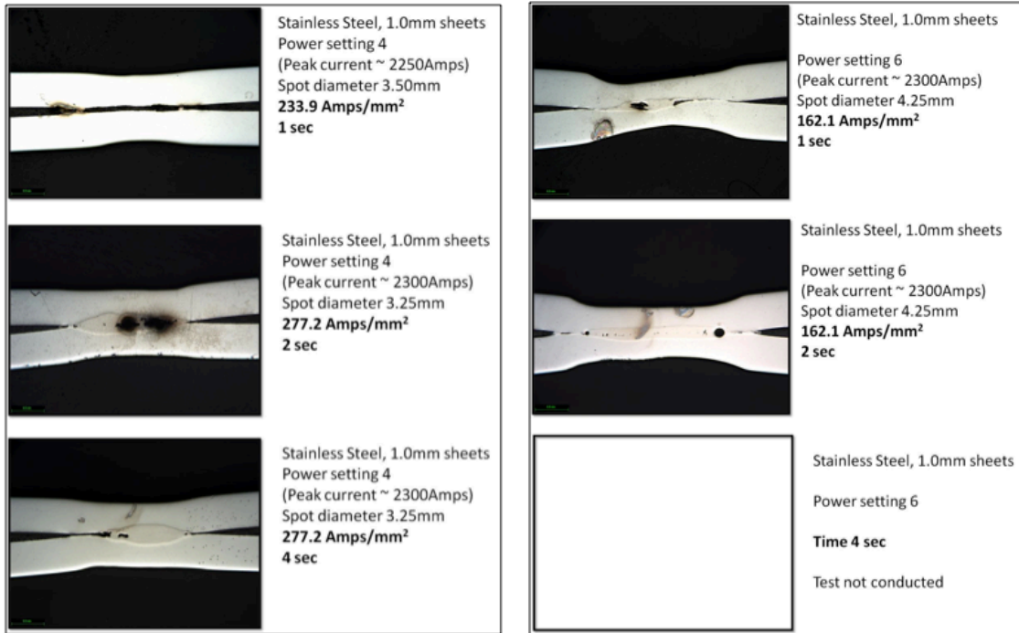
Figure 4-16 - Microsections of trials with stainless steel
