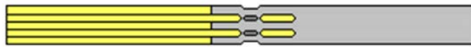
Figure 1-2 – Illustration of the metal to carbon fibre interleaved spot-weld material transition joining
