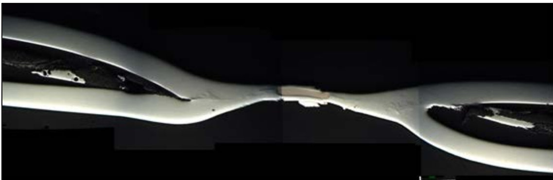
Figure 4-4 - Microsection of a preliminary trial of the hybrid material resistance spot weld concept
