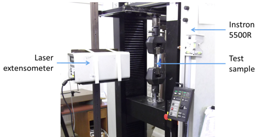
Figure 87 – Tensile test setup used for CMT Cu welded samples.
