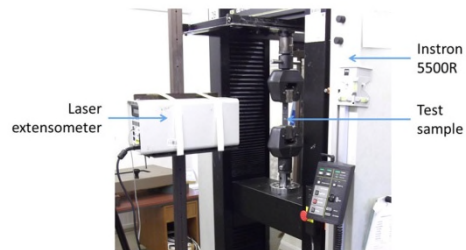
Fig. 4 Tensile test setup used for CMT Cu welded samples
