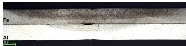
Figure 45 – Conduction mode laser spot welding macro section.
