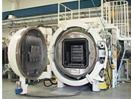
Figure 14 – Diffusion bonding chamber (Vacuum Furnace Engineering Limited, 2011).
