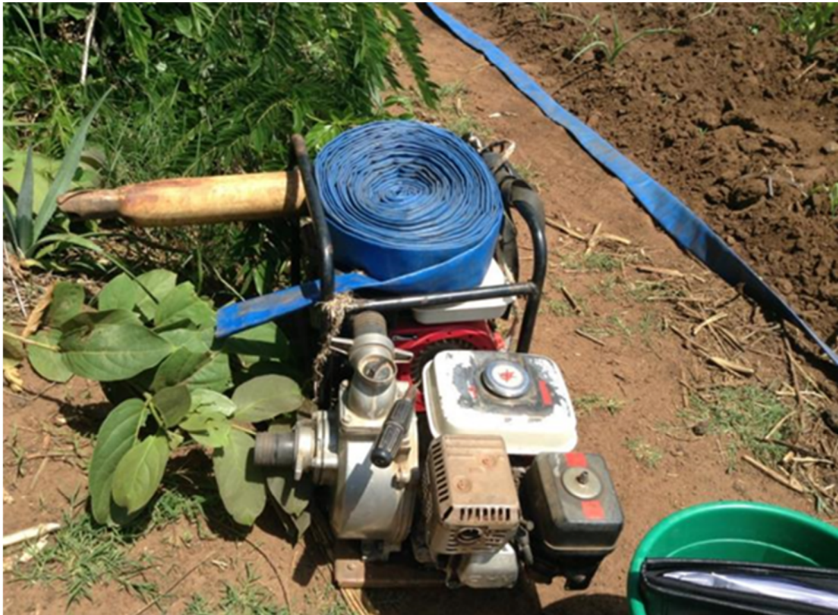
Figure 6.6: An individual motorized pump with a modified water delivery outlet (hose pipe) to match with the flexible pipes designed for the treadle pumps.
