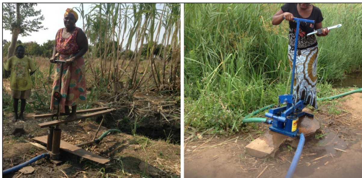
Figure 6.1: An Advait treadle pump (left) and a Money Maker pump (right) in operation at one of the irrigation sites.
