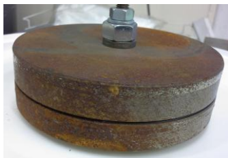
Figure 3: Surface corrosion of metal discs
