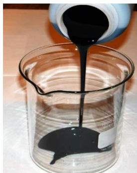
Figure 2.22: Appearance of bio-oil as a mobile dark brown liquid
