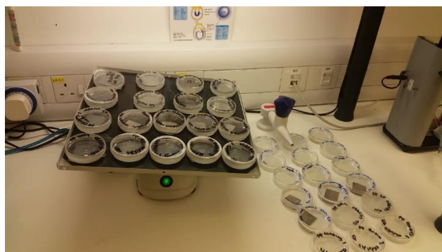
Figure.3.2.3: Long-term growth experiment set-up. Image shows example of static and non-static (rotating table) growth tests. All samples are placed directly beneath two fluorescent light tubes (15 W).
