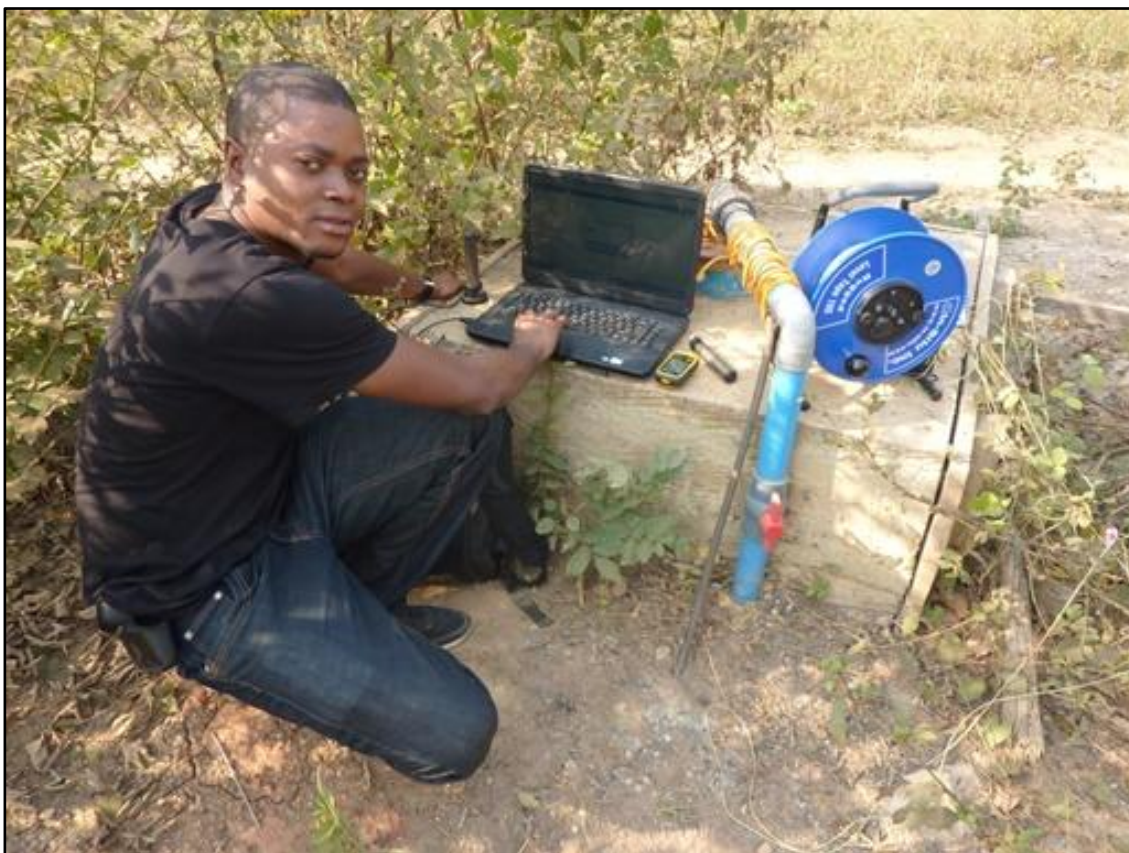
Figure 4-9: Programming and installing a water level logger
