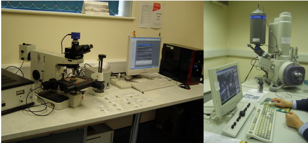
Figure 3-3 Left: Optical microscope. Right: Scanning electron microscope (SEM)
