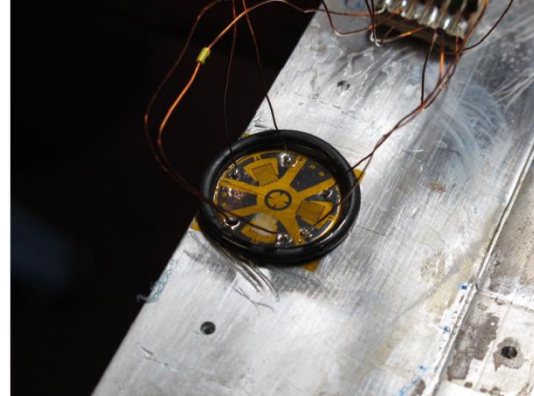
(b) Strain gauge rosette 125RE bonded
