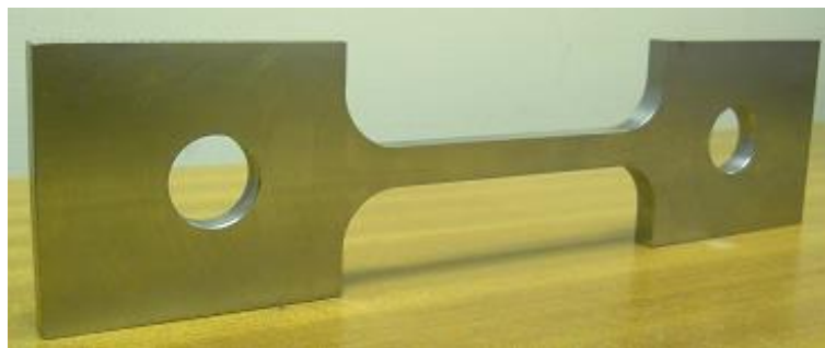
Figure 3-9 Pin-loaded tension test specimen
