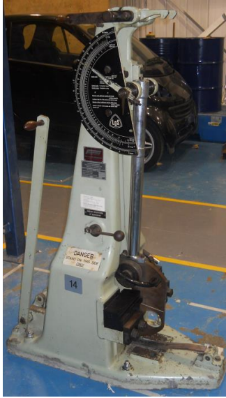
(a) Pendulum Impact tester 217 Ft-lb (~300 J) capacity
