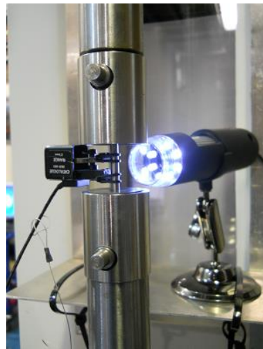
(b) 100 kN machine using round sample
