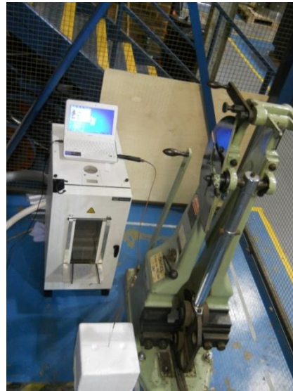
(a) Pendulum Impact tester 217 Ft-lb (~300 J) capacity
