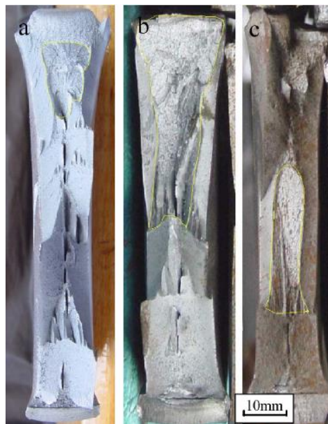
Figure 2-44 The AFAs in DWTT (a) type I, (b) type II and (c) type III [224]
