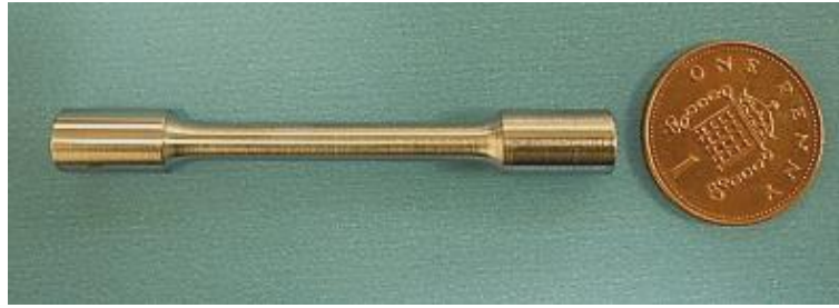
Figure 3-10 Small-size round tension test specimen
