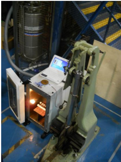
(a) Pendulum Impact tester 217 Ft-lb (~300 J) capacity
