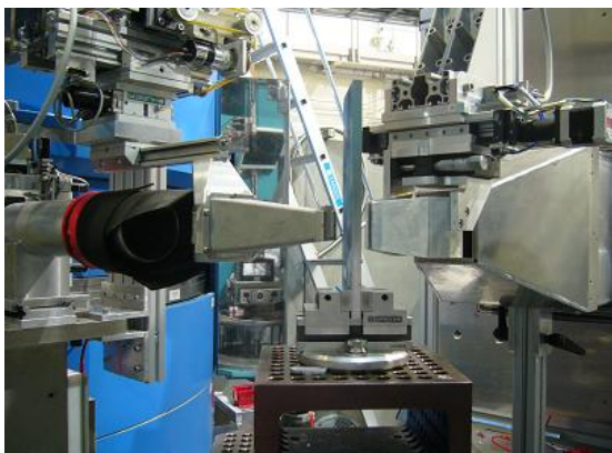
a) Set up for transverse and normal strain measurement
