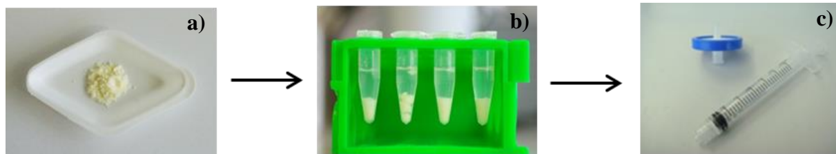
Figure 3.14 50 mg freeze dried powder (a) mixed with 1.5 mL of 50:50 (v/v) Methanol:water + 1% HCOOH (formic acid) (b) and filtered through 0.2 \mu\text{m} (c).
