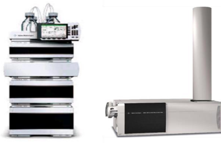
Figure 3.13 Liquid Chromatography (LC) coupled with Accurate-Mass Quadrupole Time of Flight (Q-ToF) mass spectrometer (MS) instrument.
