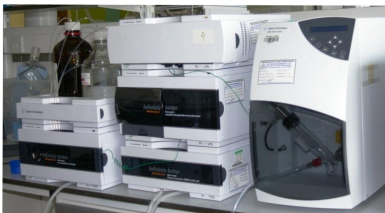
Figure 3.11 High Performance Liquid Chromatography (HPLC) Agilent 1260 series coupled to Infinity Evaporative Light Scattering Detector (ELSD) instrument.
