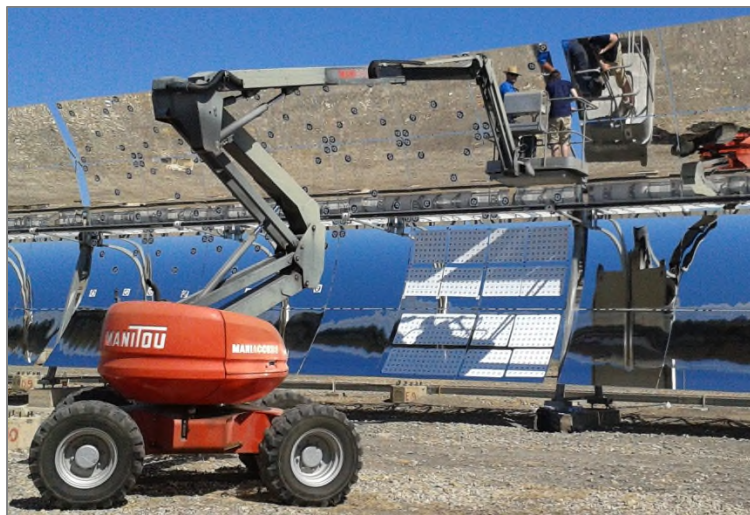
Figure 3.14 - Four facet photogrammetry at PSA
