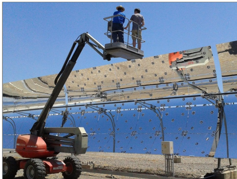
Figure 3.13 - Whole trough photogrammetry at PSA
