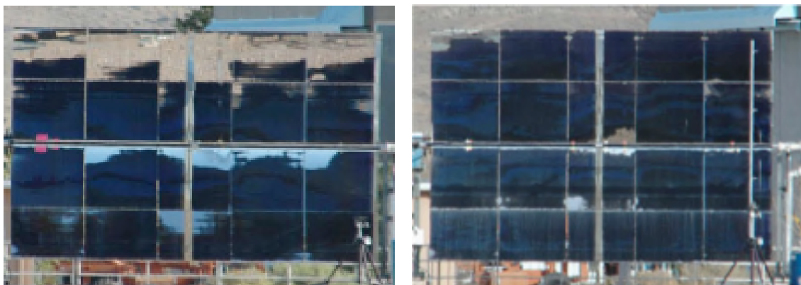
Figure 2.7 - Distant observer method, before (l) and after (r) correction
