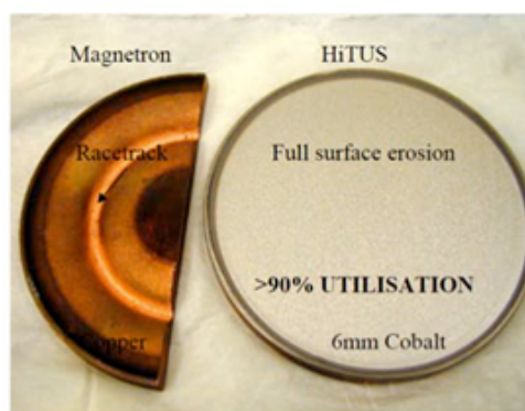
Figure 5: Magnetron v HiTUS target wear
