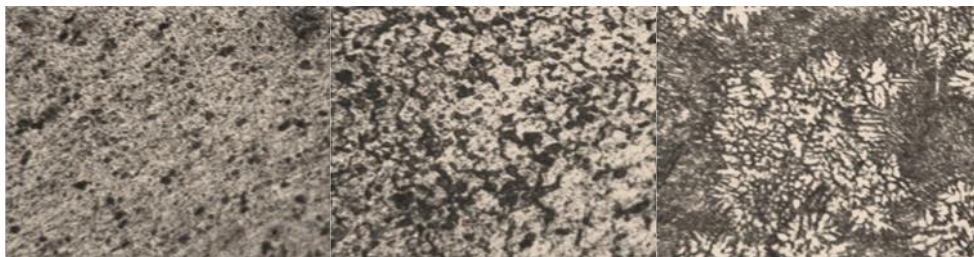
Figure 4: Optical micrographs of the different location of weld-bond a) base metal, b) heat affected zone and c) fusion zone (100X)
