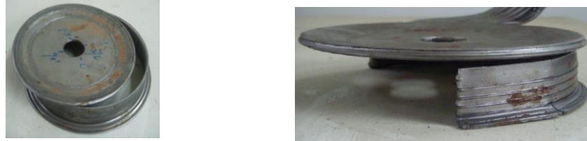
(a) bottom cutting-off during thickening (b) bottom cutting-off during tothing
