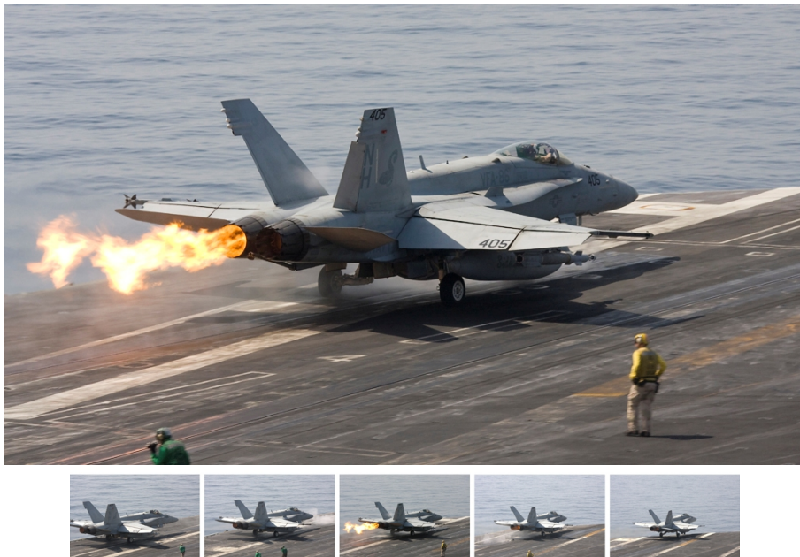
Figure 1.9: F-18C compressor surge during catapult launch - USS Nimitz 19 October 2009 [12].
