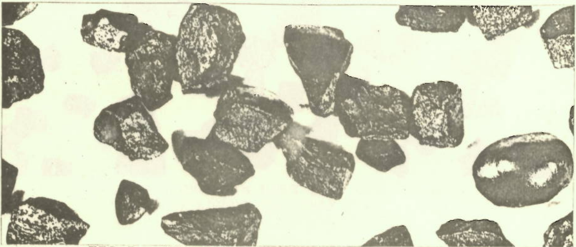
FIG. 7. NEW G39 GRIT USED FOR BLASTING OF SHIP'S HULL
