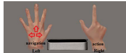
Fig. 6 Two hands' positions in relation to Leap Motion device when using Type-III hand gesture set
