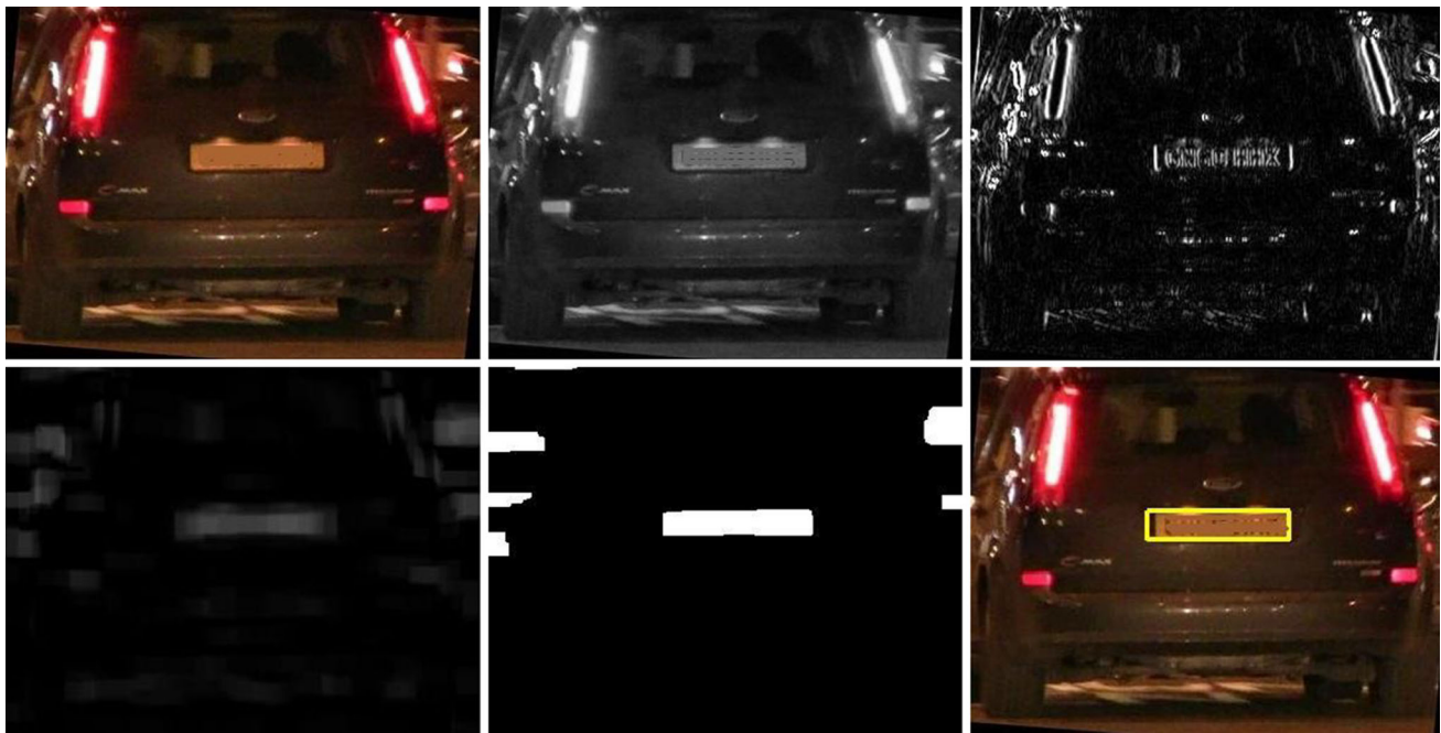
Fig. 2 License plate detection steps
