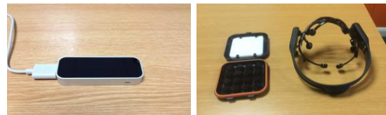
Figure 2. Peripheral devices used: Emotiv Epoc headset (right) and Leap motion controller (left).
