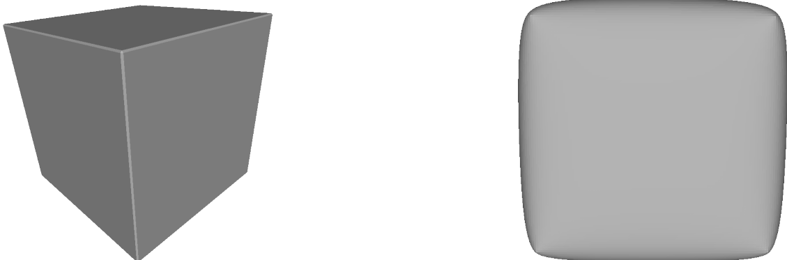
Figure 15: Left: original cube object recovered by our approach. Right: the edited cube with some of the set-theoretic operations replaced by their blended counter-parts.
