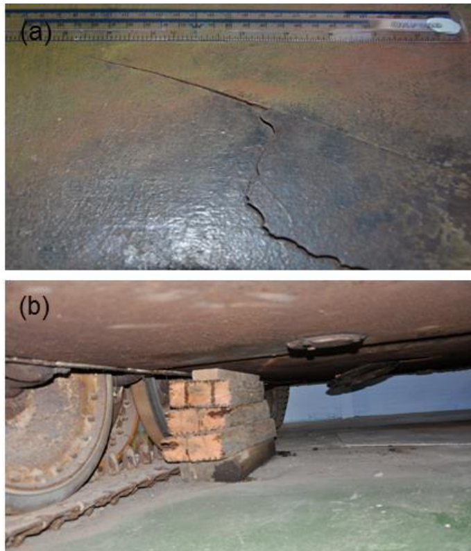
Figure 2 (a) Crack Propagation in Mark II Hull (b) Suspension Failure in Jagdpanther, sdkfz 173 [18]
