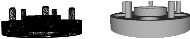
Fig. 9. A more complex CAD part recovered by our approach. Left: The input point-cloud. Right: The meshed recovered expression.
