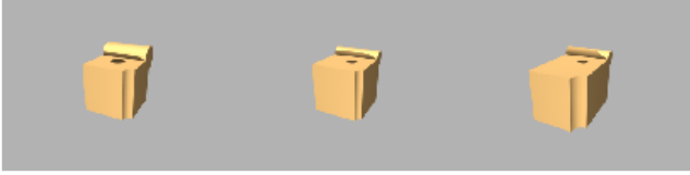
Fig. 4. Illustration of a parameterized template model: a model is built in a constructive way with abstract parameters that can be tuned to satisfy some modeling criteria.
