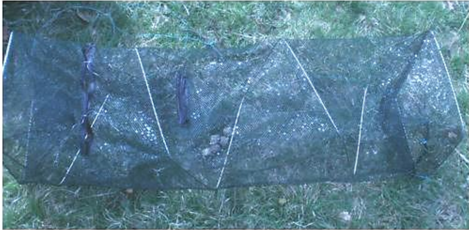
Figure 2.3 Example of the fish trap used in the study. The fishmeal pellets used as bait can be observed in the center of the trap.
