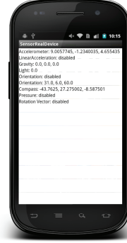
Fig. 8 Remote Mockup (RM): (left, center) A data trace of various sensor measurements encoded in JSON. The given file can be loaded to ARDs and AVDs through this subsystem; (right) An application built with SLSensorManager using the measurements.
