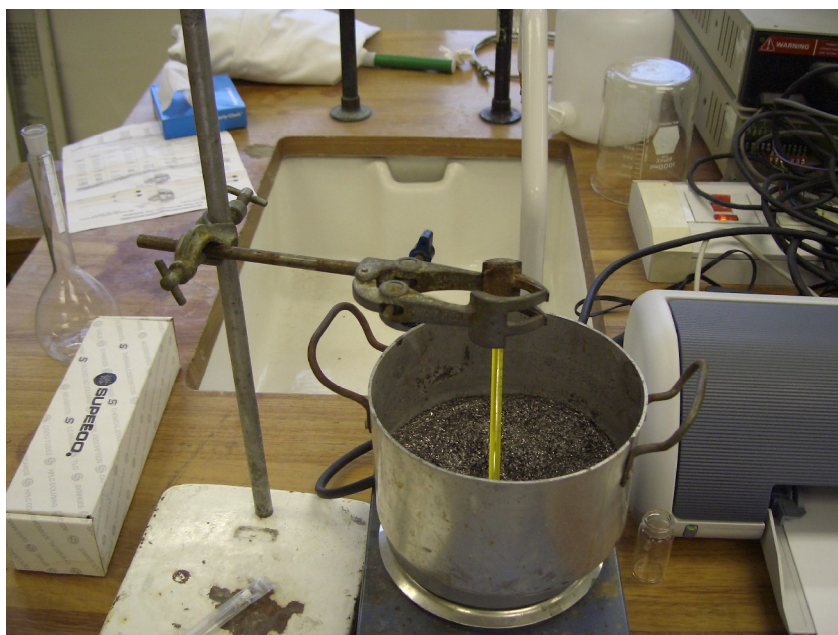
Appendix Figure 3. Carbon bath for warming essential oils to 55 °C prior to and during solid phase microextraction.
