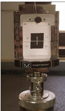
Figure 17. TBS sample glued to the grips of a tensile device.
