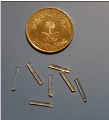
Figure 6. Bar shaped polymerized FRC.
