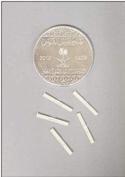
Figure 16. Bar shaped samples for TBS testing.
