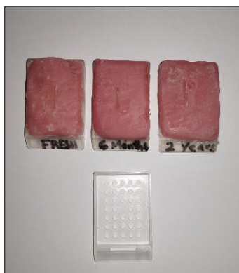
Figure 7. Tissue-processing cassettes filled with self-cured PMMA and embedded bar shaped FRC.
