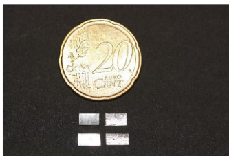
Figure 11. Rectangular shaped polymerized FRC samples bonded with resin luting material.
