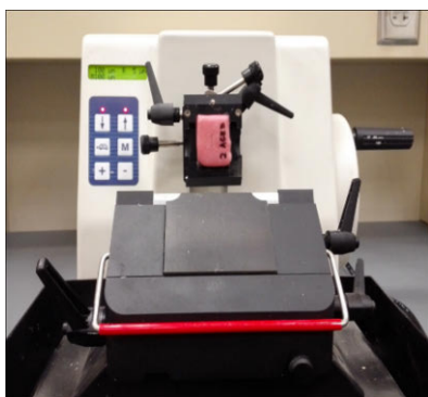
Figure 8. Longitudinal slicing of bar shaped FRC with a microtome saw.
