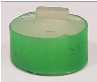
Figure 12. Study FRC sample embedded in resin luting material.
