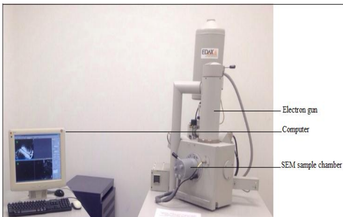
Figure 2.2: A presentation showing a scanning electron microscope (Quanta-200, FEI).
