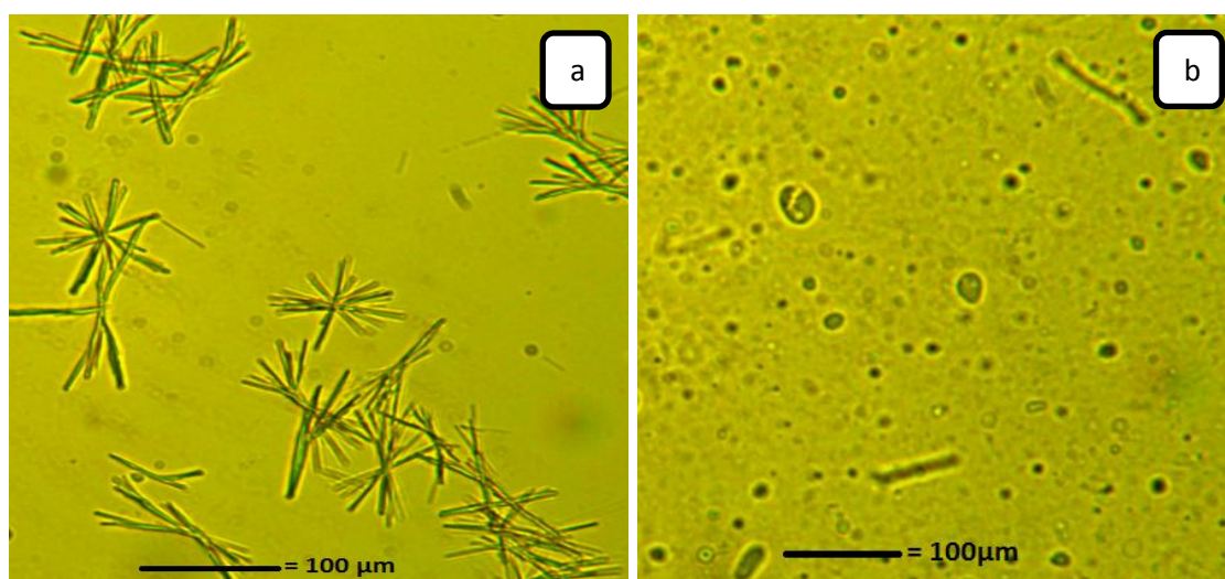
Figure 5.24: Light microscopy of (a) sedimented spot containing beclomethason dipropionate (BDP) crystals and (b) supernatant layer containing both liposome and small amount of BDP crystals, using bench centrifuge for 60 min at 13,000 rpm.
