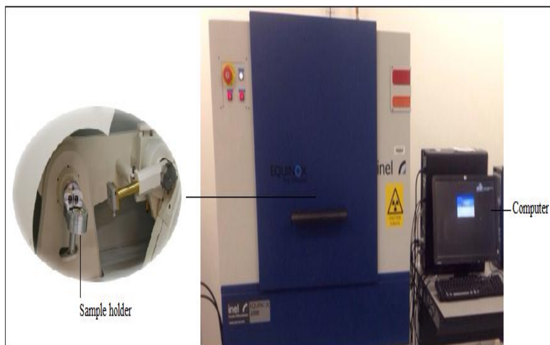
Figure 2.3: The X-ray powder diffractometer (Equinox 2000, France).
