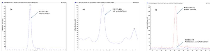
Figure 3. Example field data showing the removal of ethinylestradiol following advanced tertiary treatment. (A) Samples are collected from the WWTP following conventional (activated sludge plant) treatment following the procedures described for sample preservation. (B) Samples are extracted using solid phase extraction, cleaned-up to remove interfering substances using normal phase SPE and gel permeation chromatography. (C) The clean concentrated extract is concentrated to a low volume and analyzed using negative ion electrospray LCMS/MS in MRM mode. Results are calculated using internal standardization using isotopically labeled internal standards. In the example shown, EE2 is present in the final ASP effluent at a concentration above the predicted no effect level (PNEC) of 0.1 ng/L and is removed using GAC and ozone (O 3 ) to an environmentally safe concentration. Please click here to view a larger version of this figure.
