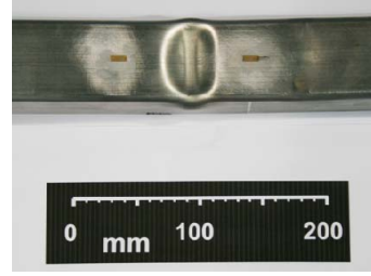
Fig. 11. Typical failure mode from 3PB tests
