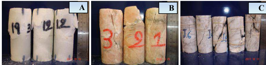
Fig. 3 The failed cylinders after short-term loading: A. the white/Bantycok gypsum. B. the pink/Bantycok gypsum. C. the Iraqi gypsum.
