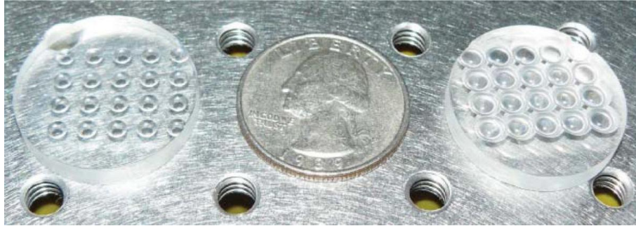
Figure 2.32 Array of concave lenses (left) and a 4×5 array of convex lenses (right)(McCall,2010)
