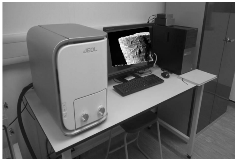
Figure 3.8 JCM-6000 NeoScope benchtop SEM (measuring cutting edge radius)
