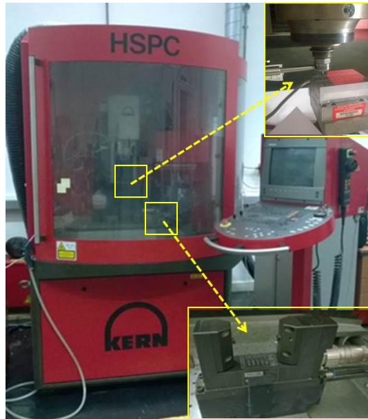
Figure 3.4 Precision micro-milling machine, cutting trial and laser measuring system (zoom-in view)
