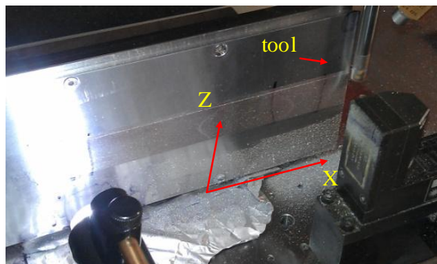
Figure 7.18 Experiment set-up for micro-milling structured surface
