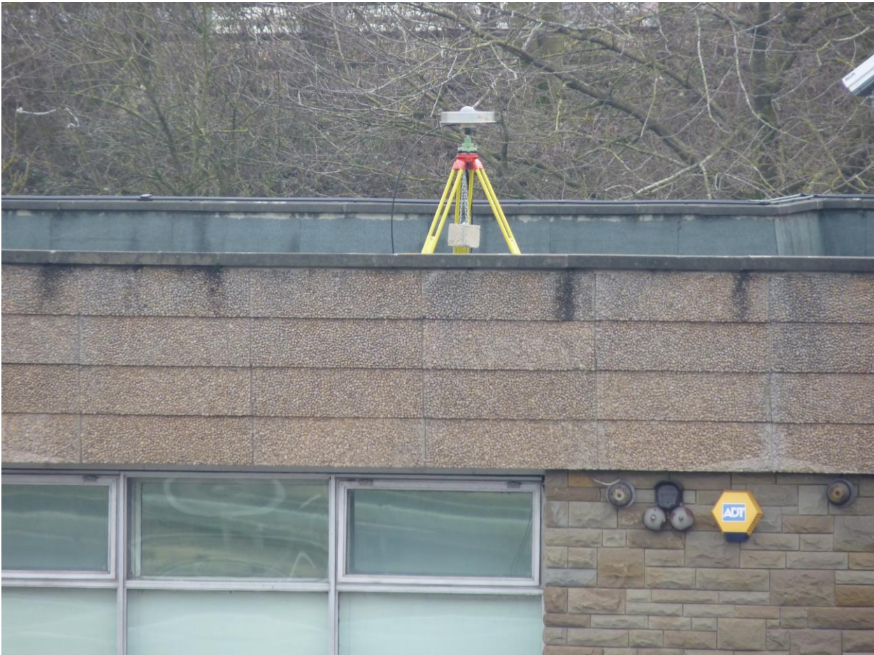
Figure 3. The principal reference GNSS antenna located upon an adjacent building to the bridge.
