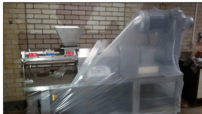
Figure 3. Screw extruder for pilot study of extrusion of fibre-cement building products
