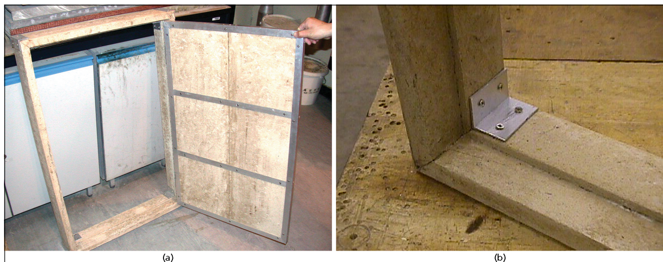
Figure 4. Extruded wood–magnesium oxychloride cement composites: (a) door frame and panels made of extruded products; (b) corner of the door with frames connected by angle steel and nails
