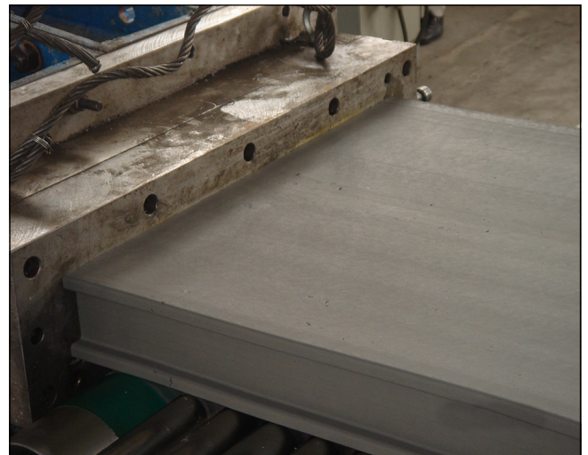
Figure 7. Fibre-cement extrudate just after die-exit
