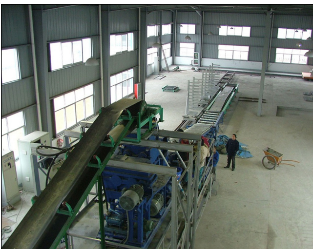
Figure 6. Overview of fibre-cement building products extrusion factory
