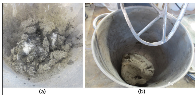
Figure 1. Semi-solid, dough-like fresh cement-based materials for extrusion: (a) during mixing not suitable for extrusion; (b) suitable for extrusion
