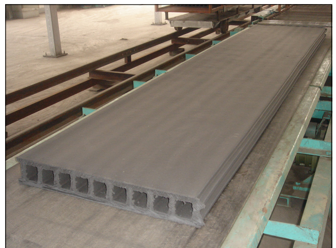
Figure 8. Extruded honeycomb fibre-cement partition wall panel of 600 mm x 90 mm cross-section and several metres long
