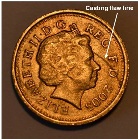
Fig. 1 Counterfeit £1 coin with casting defect.
