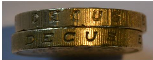
Fig. 3 Counterfeit £1 coin (top), compared to a genuine coin (bottom), has poor quality edge milling and lettering.
