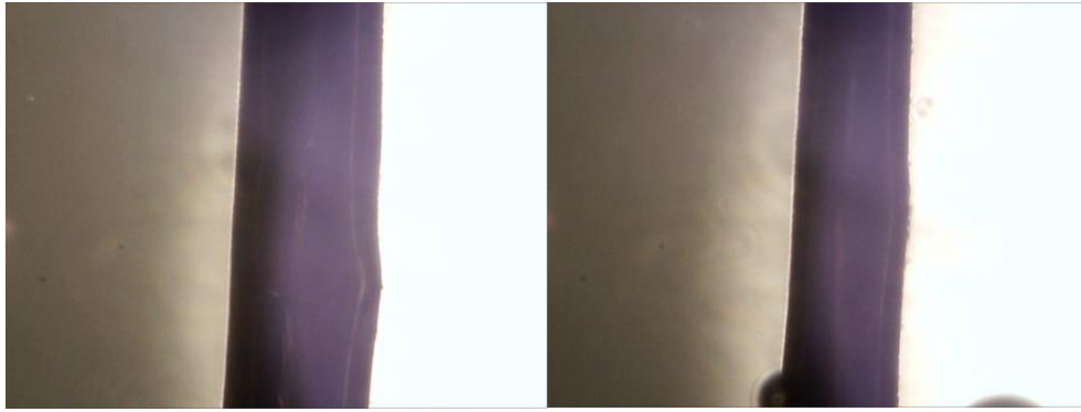
Figure 2.22. A probe shown in two different stages of etching. The difference of the diameters can be used as an alternate indication of the material removed. Left: Width of probe before 1350s: 265 \mu m Right: Width of probe after 1600s: 204 \mu m
