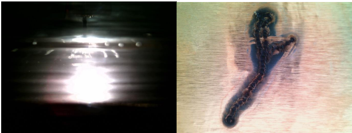
Figure 4.19. Left: The larger plasma region, the 0.25 mm wide tungsten probe can be seen in the centre top of the image. Right: the random motion of the arc assembled thread due to fluidic motion is seen leaving arc-eroded marks on the protective copper tape.
