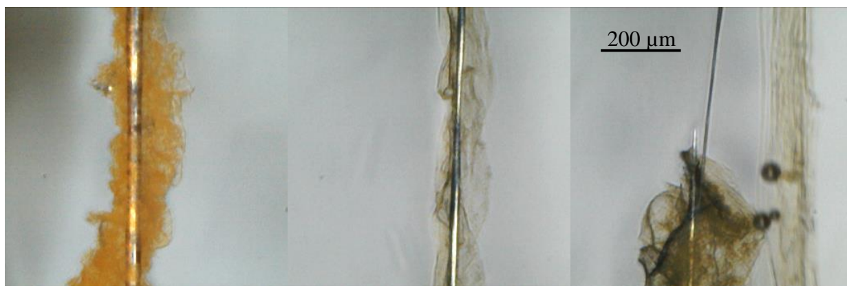
Figure 2.13. Three images showing \text{WO}_3 formation and progression to probe collapse.
