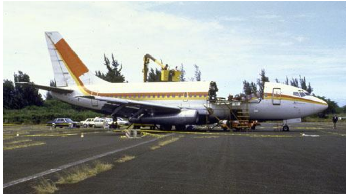
Figure 1.1: Damaged Aloha airline flight 243 [1]
