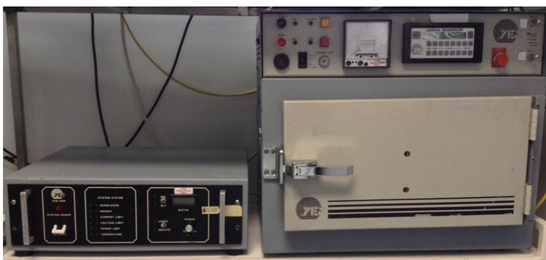
Figure. 3.8. YES-R3 oxygen plasma etching system.
