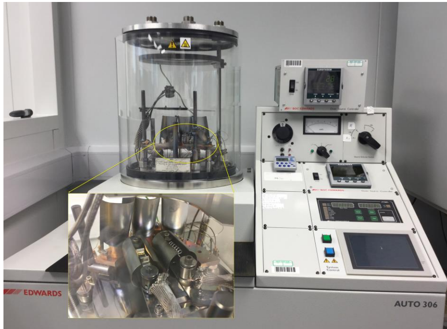
Figure. 3.10. Photograph of an Edwards Auto 306 evaporator.
