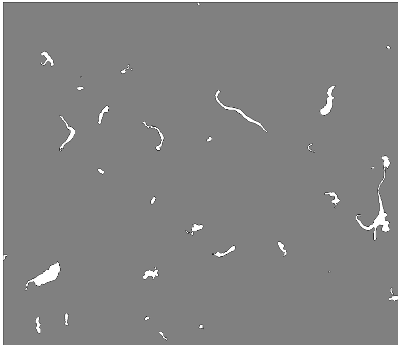
Figure 4.7 Segmented image of UHMWPE particles obtained after watershed segmentation. White regions are the segmented particles. Each particle is outlined by a thin black boundary. Gray region is the background.
