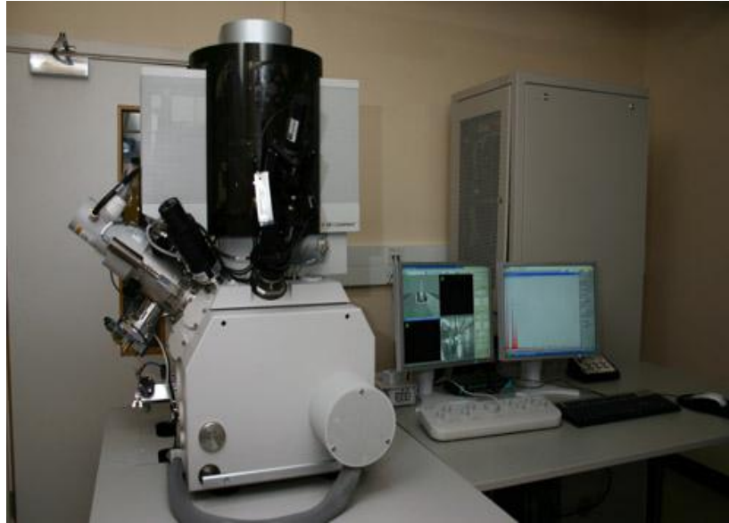
Figure 3.19 FEI Helios Nanolab™ 600 scanning electron microscope used for SEM imaging in the current study.
