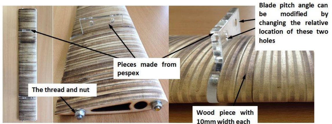
Figure 6.7 Photograph of the H-Darrieus blade showing threads, nuts, wood laminates and perspex mounting pieces. Pre-set blade pitch angle can be modified by replacing perspex pieces with different relative hole locations.
