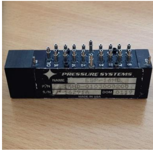
Figure 6.14 The 16-channel miniature pressure scanner ESP-16HD.
