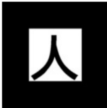
Figure 2.2: An Example Fiducial Marker from the ARToolkit Project (Kato and Billinghurst (1999)) showing subtle asymmetry
