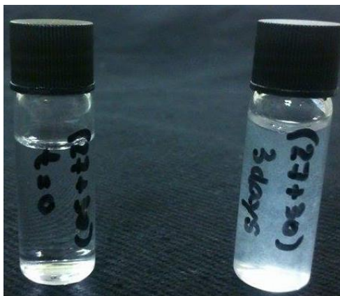
Figure 4.15: Visual comparison of 100 \mu\text{M} solutions of (SAF+c-3PAL14) ( 27+30 ) in 10 mM MOPS buffer at pH 8.5 at 21 ^{\circ}\text{C} at different times of their maturing process: just prepared sample at the left hand side vs a three-days old sample.
