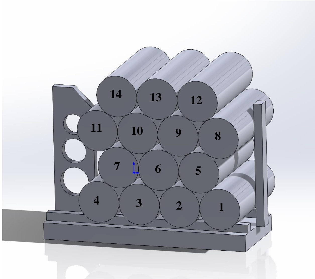
Figure 27: Billet Rack with labeled billet positions
