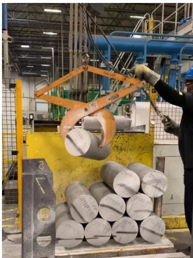
Figure 1. Extrusion process operator loading billet into oven.
