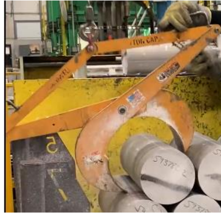
Figure 9: UAC’s current solution for picking up billets.
