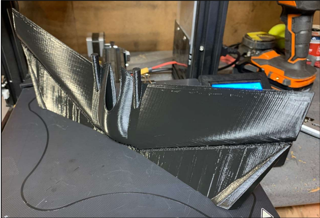
Figure 96: Wind Tunnel Test Model V2 Printed with Tree Supports
