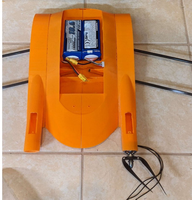
Figure 104: 3-D Printed Aircraft Body Displaying a mounted Motor and Battery Fit.
