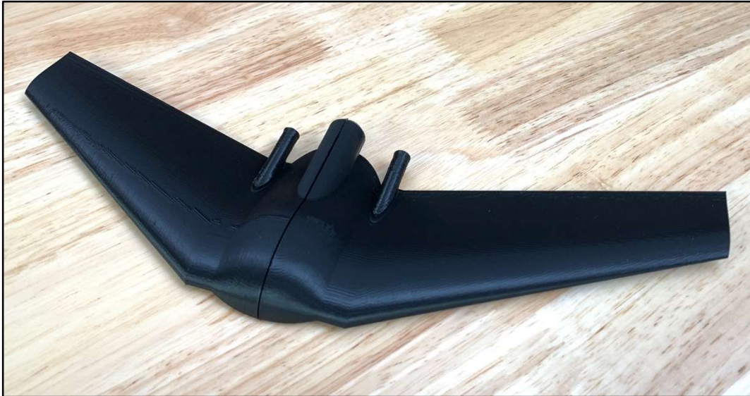
Figure 95: Wind Tunnel Test Model V1
