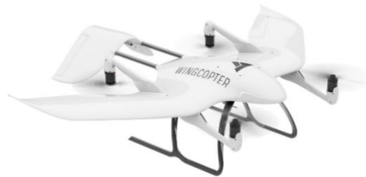
Figure 3: Wingcopter Tilt-Rotor Quadcopter Design [9]
