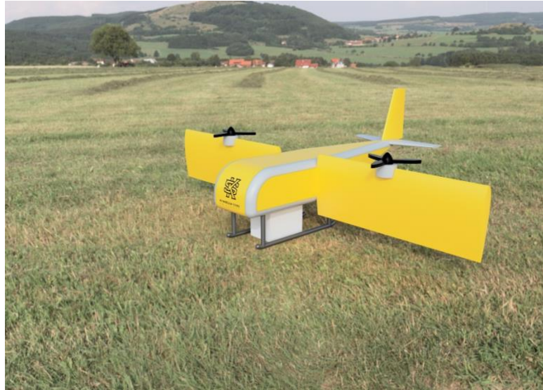
Figure 30: Final CAD Render in Helicopter Mode with Package Lowered
