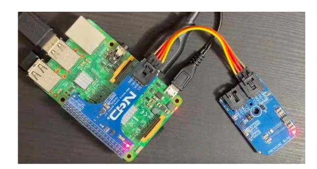
Fig: Prototype consist of Raspberry Pi4 connected to a BMP180 pressure sensor that transfers the data using a 12C Shield digitizer.
