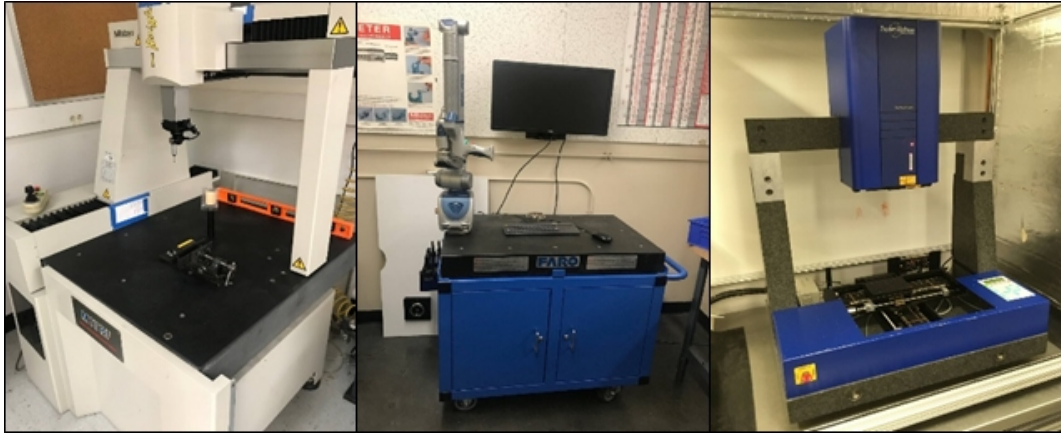
■ Figure 2 Mitutoyo Bright BRT 504 - tactile CMM (left), Faro Arm Edge and Scan Arm HD - Laser line and tactile probe CMM (middle), and Taylor Hobson Talyscan 250 - Laser triangulation CMM (right).
